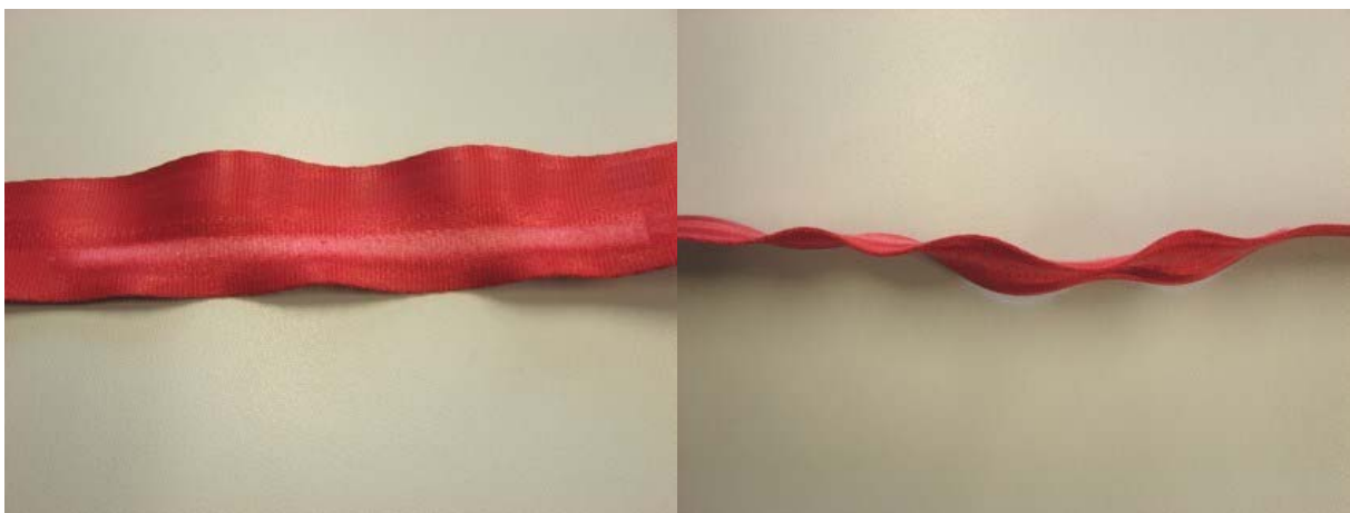
Illustration 5-5: Unacceptable Webbing Wear
